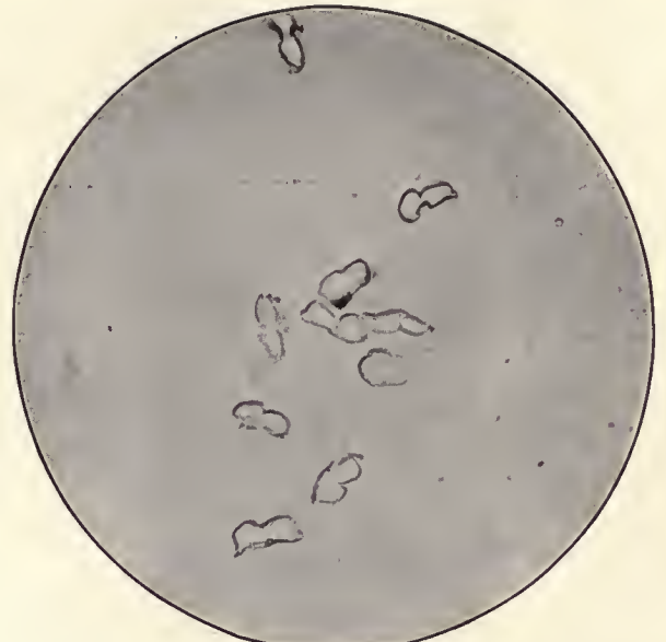
FIG. 2.—RAW SILK. Bombyx mori . Single fibres in transverse section showing each fibre or "bave" as dual cylinder. \times 235 .
